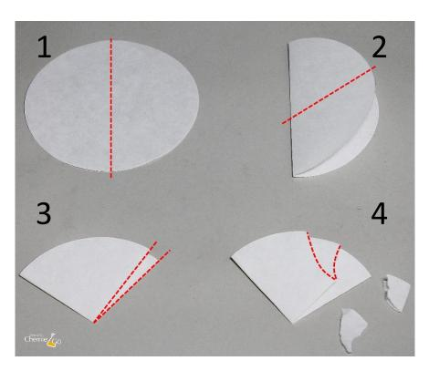
One important aspect to correctly use an analytical funnel is to correctly fold the filter.
