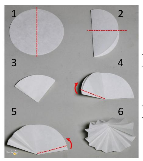
If no folded filter is available, a filter paper disk can be folded following the displayed procedure.
