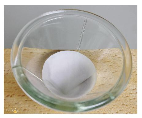
Special filters are used for analytical work. They have a defined ash content and are incinerated with the residue. The ash content is stated on the packaging.
